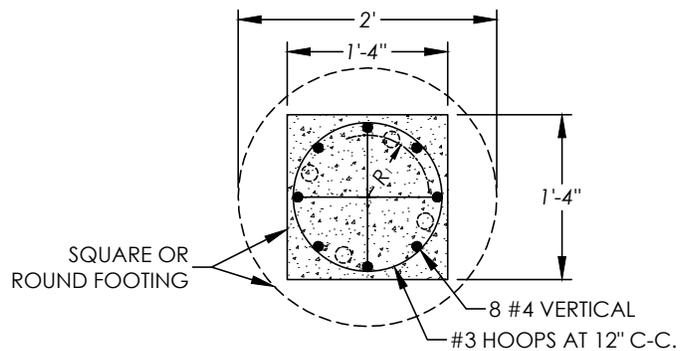
R<sub>1</sub> = ANCHOR BOLT DIA. DIMENSION R AND
